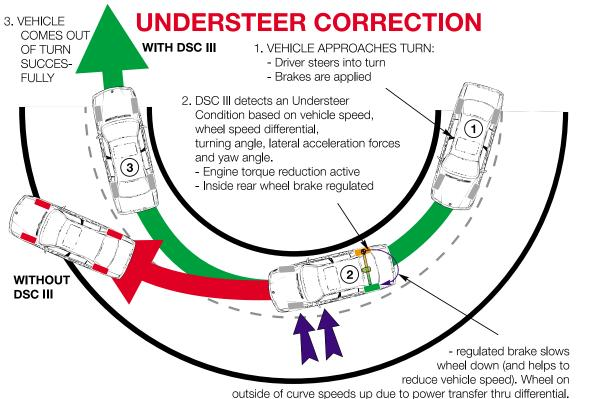
Vehicle pivots in favor of curve. Combined, this forces the vehicle into the turn.
